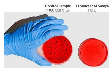
Sample Log Reduction Test (Comparing CFU (Colony Forming Units), Before & After)
