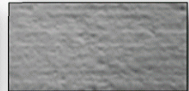
CSP 4 (light scarification)
